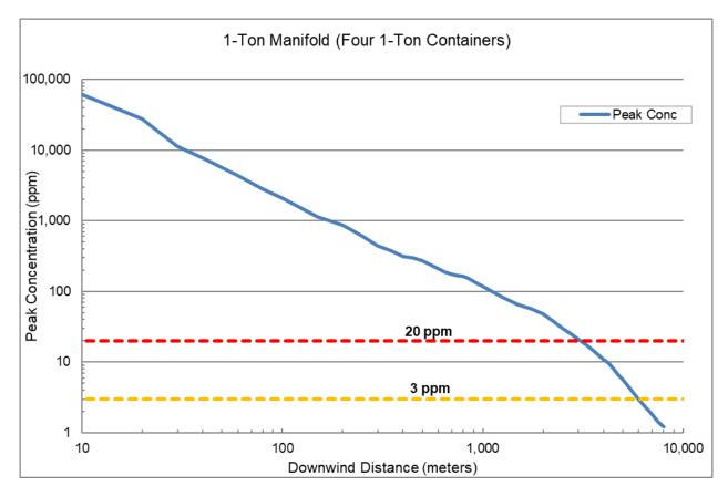
5.2.4 Alternative-Case 1-Ton Manifold (Four 1-ton Containers) Scenario – D Stability
