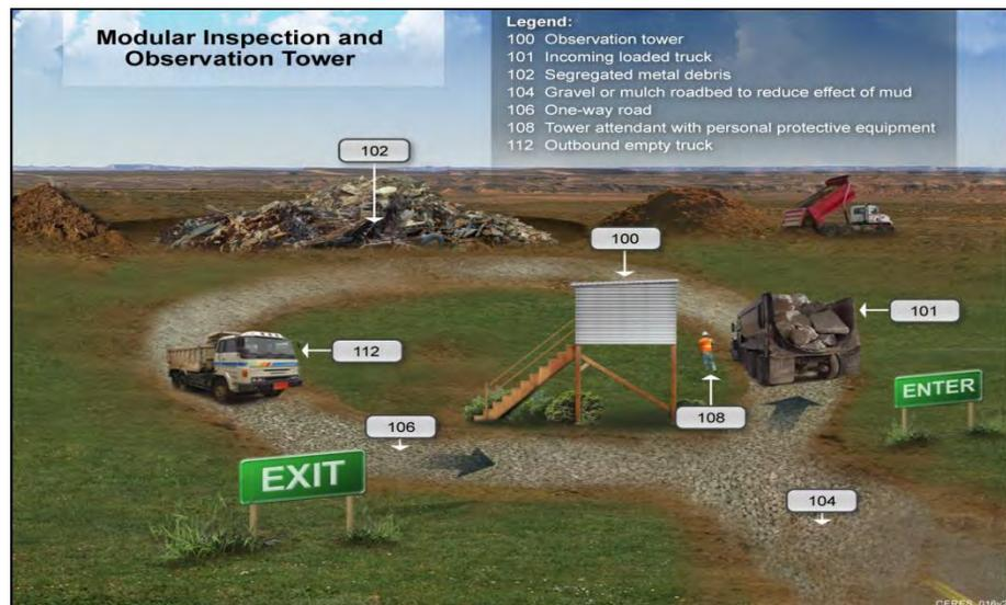
the truck and estimated load volume (percent capacity) and evaluate the load for contaminants requiring separation. The Monitor will instruct the driver regarding the appropriate dump location at the site and will verify the truck is completely empty following dumping. The Monitor will complete the load ticket presented for each load delivered to the site.
