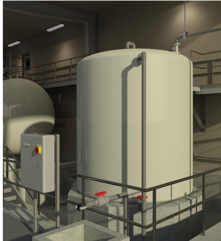
▲ 3D design of chemical bulk storage using BIM rendering
