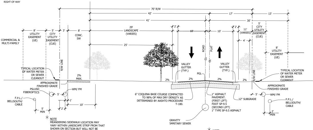
70' RIGHT-OF-WAY TYPICAL SECTION POSTED SPEED 25 MPH
