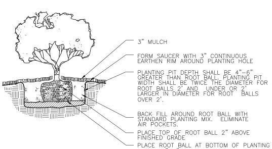
PIT ON 4"-6" LAYER OF COMPACTED STANDARD PLANTING MIXTURE
