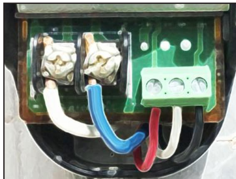
Ped Call Wires/Terminal on Left. 3-Position Terminal Block on right (for operating as iN3)
