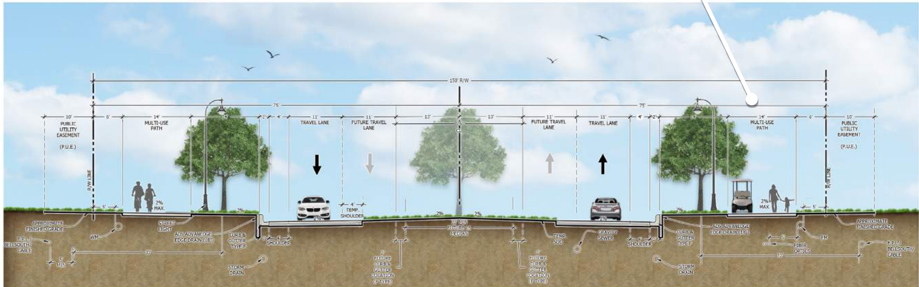
N/S A 150' ROW TYPICAL ROADWAY CROSS SECTION
