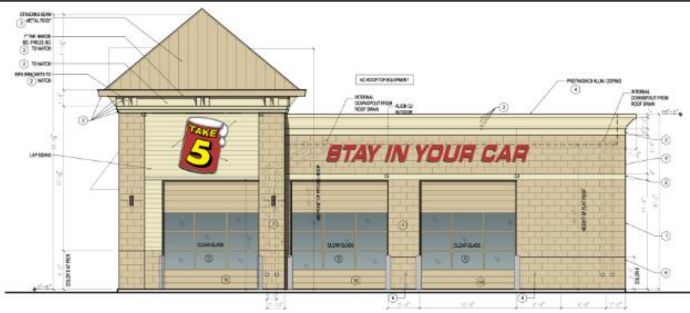
1 NORTH ELEVATION SCALE: 1/4" = 1'-0"
