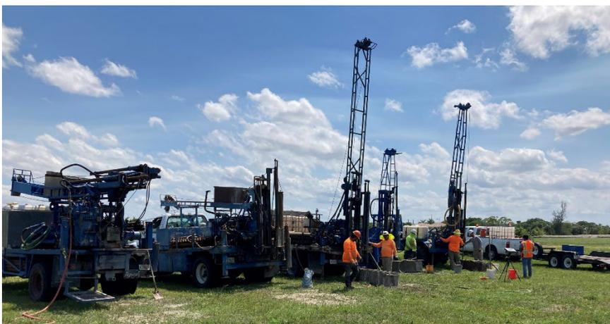
The CME 550 Mudbug and Diedrich D-25 Track rigs can perform Standard Test Borings (SPT) for depths up to 150 feet. This rig allows access on projects where site conditions consist of soft or wet surface conditions. This rig can also be utilized in areas with up to 18 inches of standing water.
