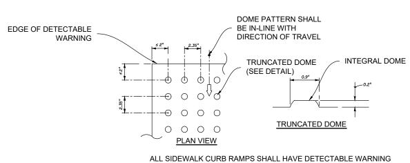
SURFACES THAT EXTEND THE FULL WIDTH OF THE RAMP AND IN THE DIRECTION OF TRAVEL 24 INCHES (610 MM) FROM THE BACK OF CURB
