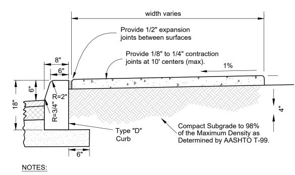
1. USE 3,000 P.S.I. CONCRETE AT 28 DAYS FOR CONSTRUCTION. 2. SUBGRADE TO EXTEND AN ADDITIONAL 6" BEYOND TYPE "D" CURB.
