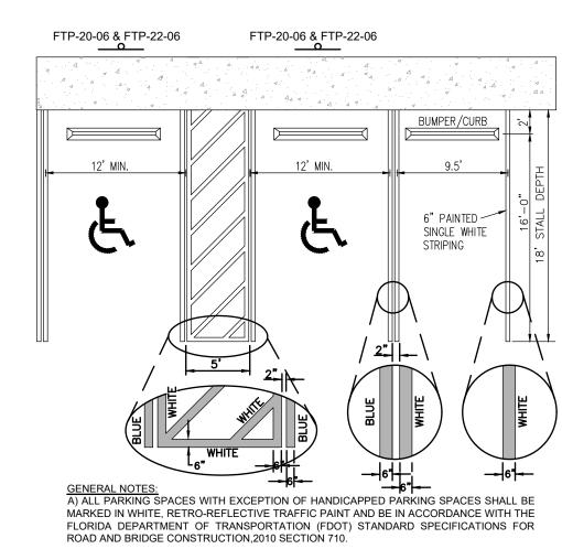
B) ALL HANDICAPPED PARKING SPACES SHALL BE PROPERLY SIGNED AND STRIPED IN ACCORDANCE WITH THE FDOT STANDARD INDEX 17346, FY 2017-18. C) ALL COMPACT SPACES SHALL BE MARKED "COMPACT" ON THE STALL OR TIRE STOP.
