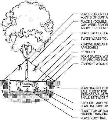
PLACE RUBBER HOSE ON WIRE AT ALL POINTS OF CONTACT WITH TREE
