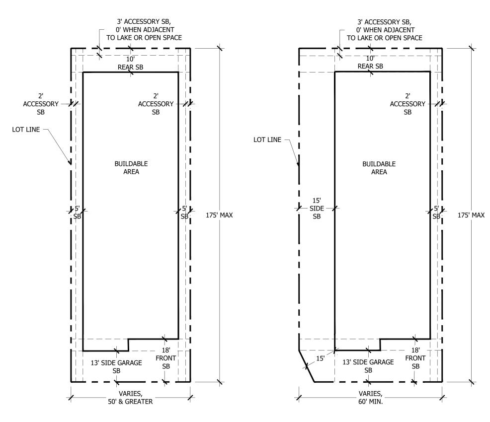
WIDTH OR GREATER, THE SIDE CORNER LOT SETBACK CAN BE REDUCED TO 5'. WHEN NOT ADJACENT TO AN OPEN SPACE TRACT, SIDE SETBACK SHALL BE A MINIMUM OF 10' ON STREET SIDE.
