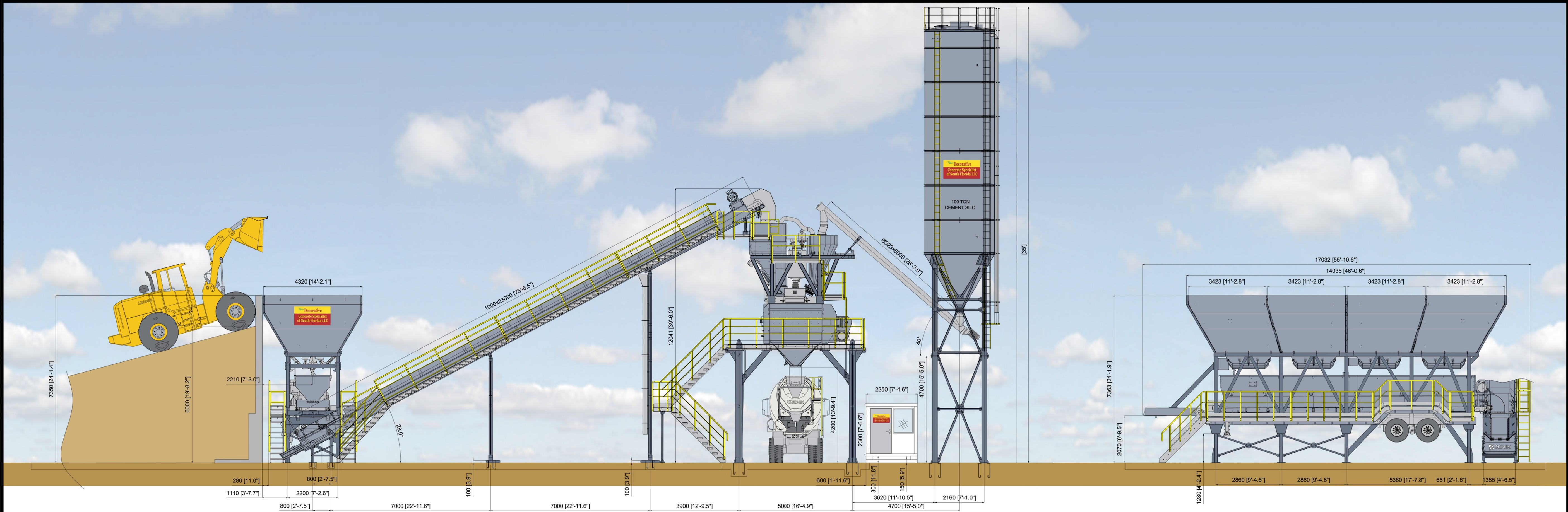
PROPOSED AGGREGATE BATCHER & SILO DETAIL
