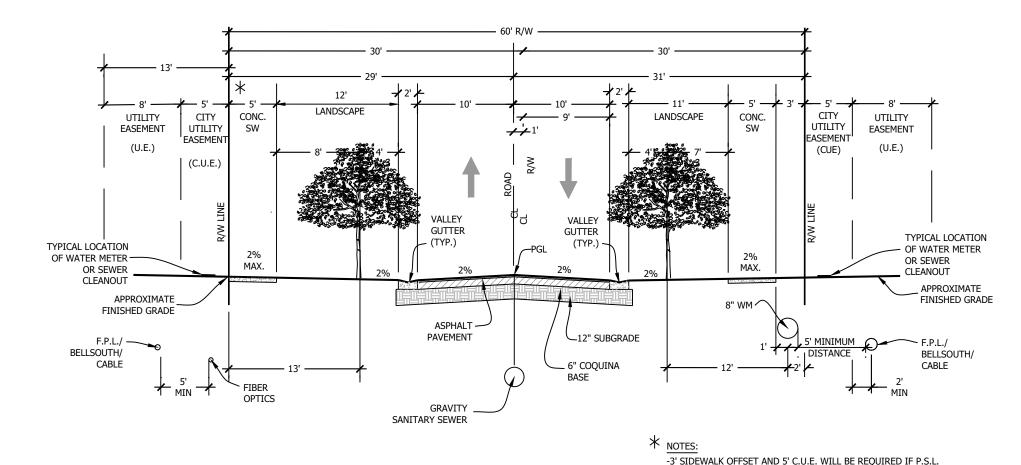
60' RIGHT-OF-WAY TYPICAL SECTION POSTED SPEED 25 MPH
