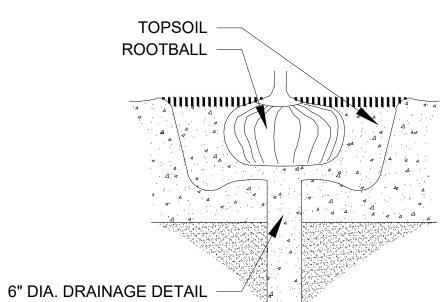
DRAINAGE TESTING DETAIL
