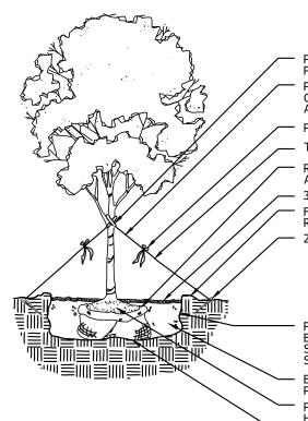
PLACE RUBBER HOSE ON WIRE AT ALL POINTS OF CONTACT WITH TREE - PLACE 3 (DOUBLE STRANDS) 12 GAUGE GALVANIZED GUY WIRE, SPACED EQUAL DISTANCE AROUND TREE ABOVE FIRST LATERAL BRANCH - PLACE SAFETY FLAGS ON GUY WIRES – TWIST WIRES TO ADJUST TENSION ON GUY WIRE - REMOVE BURLAP FROM TOP 1/3 OF ROOTBALL IF APPLICABLE — 3" MULCH FORM SAUCER WITH 4"-6" CONTINUOUS EARTHEN RIM AROUND PLANTING HOLE 2"x4"x24" WOOD STAKE DRIVEN 3" BELOW GRADE
