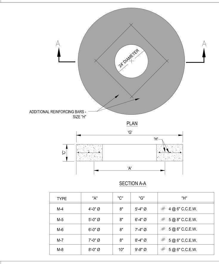
5 PRECAST CONCRETE-TOP SLAB FOR DRAINAGE MANHOLES
