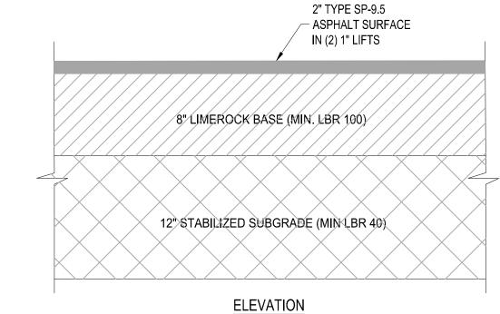
ASPHALT PAVEMENT DETAIL SCALE: NONE
