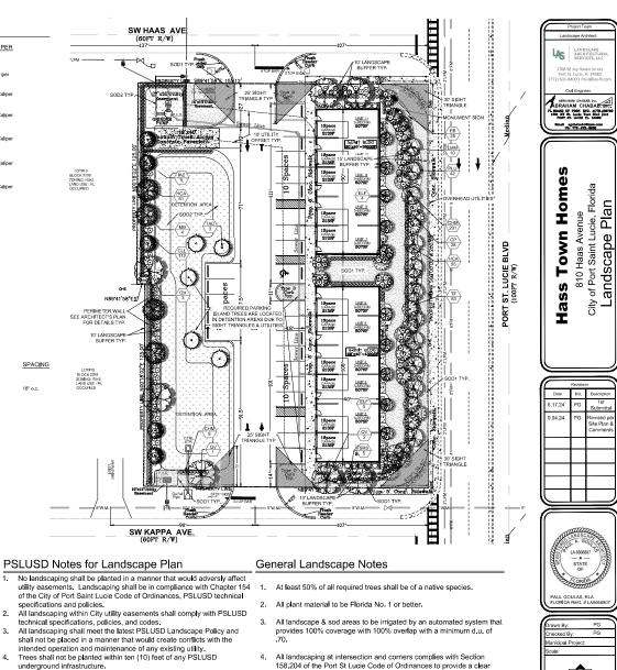
5. No landscaping other than sod grasses shall be located within 5' of a PSLUSD appurtenance such as a water meter assembly, backflow device, fire hydrant, or sewer cleanout, etc.
