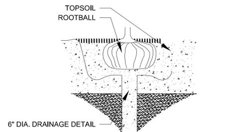
**DRAINAGE TESTING DETAIL**
