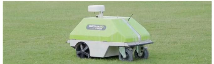
This reduces the amount of staff time that is required to perform the task, while also saving on the amount of paint used. As an example, when the Turf Tank is used to paint soccer fields it saves an estimated 8-10 hours of staff time. That allows the parks staff to complete other necessary projects while the technology gets the job done.
