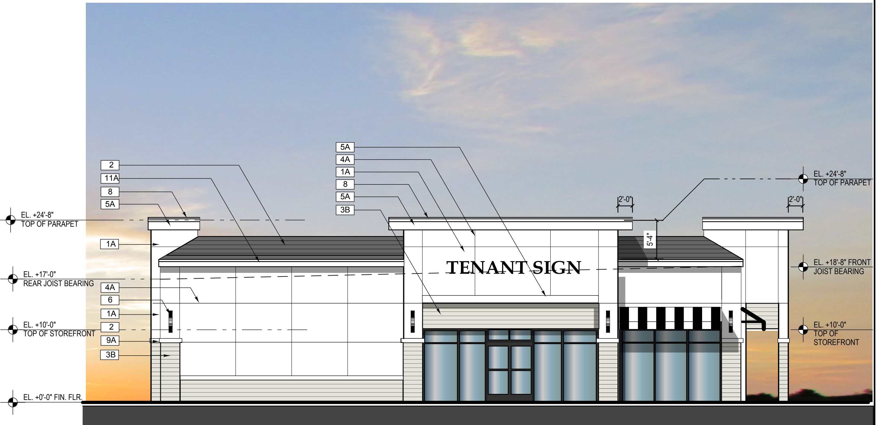
○ RETAIL SIDE ELEVATION (NORTH) 1/8" = 1'-0"
