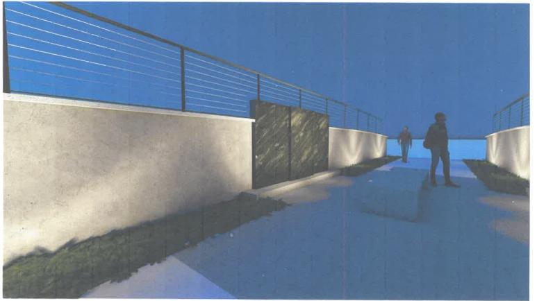
\* Lucido Design recommendation, 6 panels, 3 each side of walkway, affixed to the cement walls, with metal wire fencing across the top of each panel.
