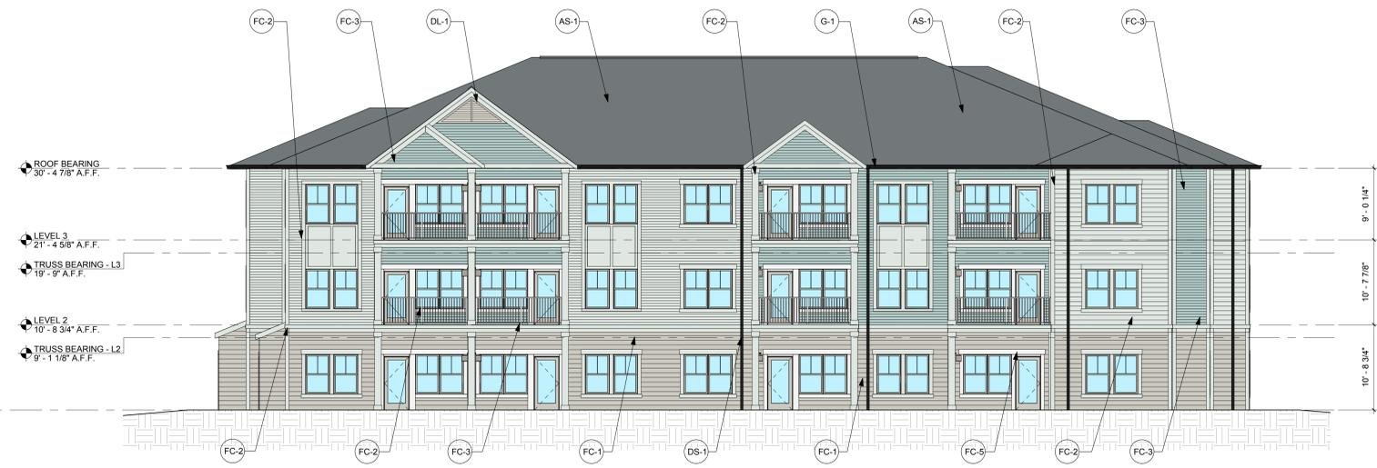
4 BUILDING 'TYPE A' - REAR ELEVATION COLOR SCALE: 1/8" = 1'-0"
