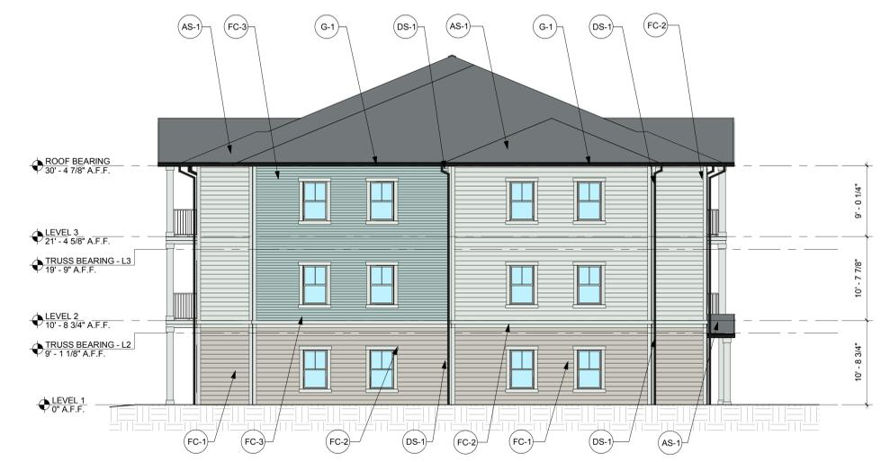
3 BUILDING 'TYPE A' - LEFT SIDE ELEVATION COLOR SCALE: 1/8" = 1'-0"
