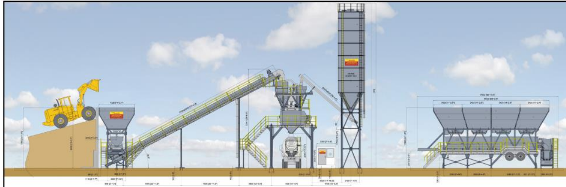
PROPOSED AGGREGATE BATCHER & SILO DETAIL
