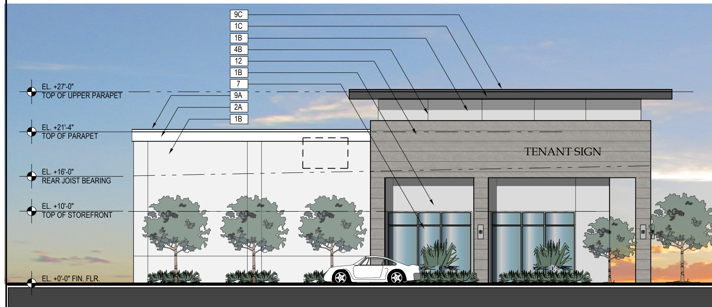
SIDE ELEVATION BUILDING #1 & #2 1/8" = 1'-0"
