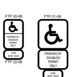
1. FTP 20-06: TOP PORTION SHALL HAVE REFLECTIVE BLUE BACKGROUND WITH WHITE REFLECTIVE SYMBOL AND BORDER. BOTTOM PORTION SHALL HAVE A REFLECTIVE WHITE BACKGROUND WITH BLACK OPAQUE LEGEND 2. FTP 21-06: TOP PORTION SHALL HAVE REFLECTIVE BLUE BACKGROUND WITH WHITE REFLECTIVE SYMBOL AND BORDER. BOTTOM PORTION SHALL HAVE A REFLECTIVE WHITE BACKGROUND WITH BLACK OPAQUE LEGEND AND BORDER. 3. FTP 20-06 IS FOR USE IN AREAS WHERE SPACE IS LIMITED.
