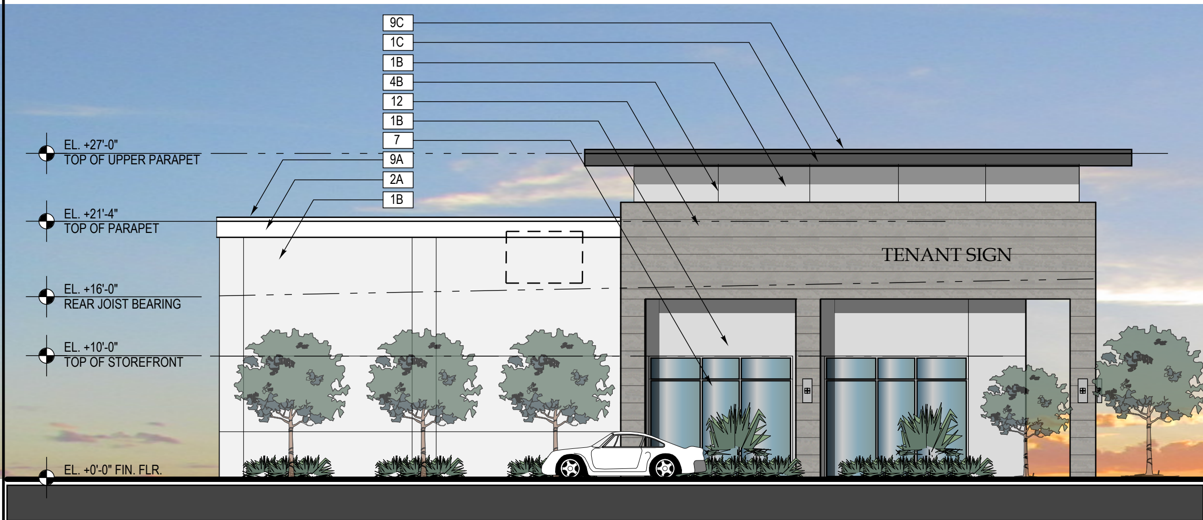
SIDE ELEVATION BUILDING #1 & #2 1/8" = 1'-0"
