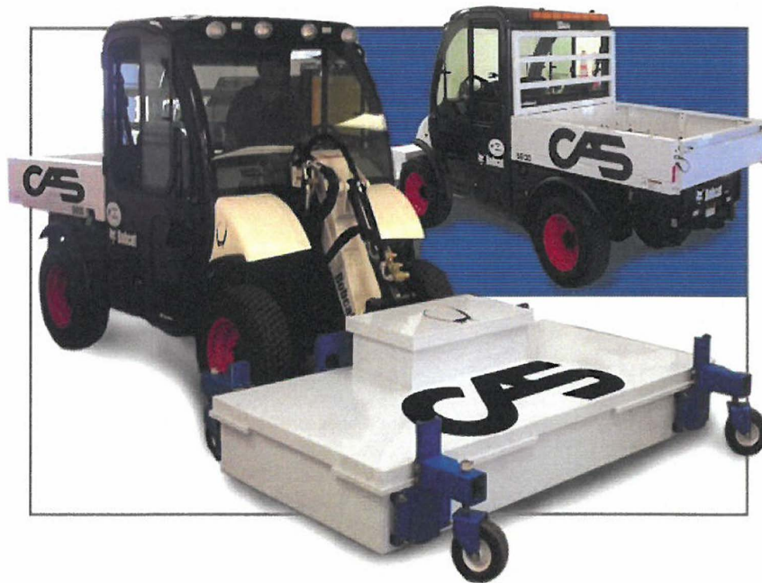
Typical 3-D Radar Tomography Scanning Unit
