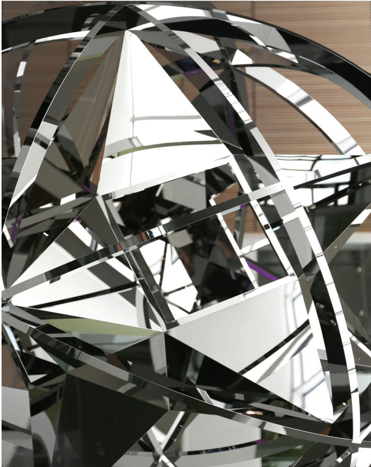
The mobile for the very core of the VIA school building is an assembly of five spherical objects attached to a steel structure consisting of four horizontal tiers and vertical hanging pipes of various dimensions. Each of the spheres has one LED illuminated ring. The intensity of the illumination varies from sphere to sphere.
