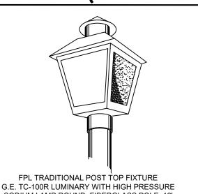
SODIUM LAMP ROUND, FIBERGLASS POLE, 12' HEIGHT (BURY 5' IN DEPTH).
