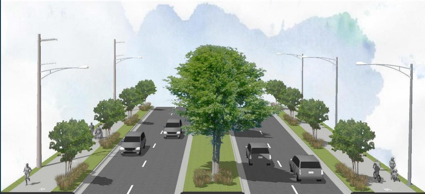
Typical Section of Port St. Lucie Blvd. Planned Condition for Port St. Lucie Blvd. South
