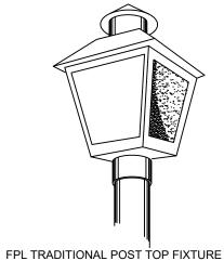
G.E. TC-100R LUMINARY WITH HIGH PRESSURE SODIUM LAMP ROUND, FIBERGLASS POLE, 12' HEIGHT (BURY 5' IN DEPTH).
