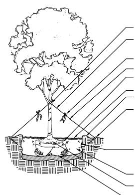
PLACE RUBBER HOSE ON WIRE AT ALL POINTS OF CONTACT WITH TREE PLACE 3 (DOUBLE STRANDS) 12 GAUGE GALVANIZED GUY WIRE, SPACED EQUAL DISTANCE AROUND TREE ABOVE FIRST LATERAL BRANCH PLACE SAFETY FLAGS ON GUY WIRES - TWIST WIRES TO ADJUST TENSION ON GUY WIRE - REMOVE BURLAP FROM TOP 1/3 OF ROOTBALL IF APPLICABLE - 3" MUI CH
