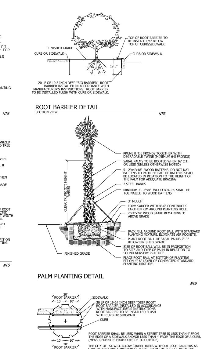
THE CITY OF PSL WILL ALLOW STREET TREES WITHOUT ROOT BARRIERS AS LONG AS THEY ARE A MINIMUM OF 4 FEET FROM THE EDGE OF BOTH THE SIDEWALK AND CURB. THIS MEANS THE TREE LAWN MUST BE NO LESS THAN 8'. ROOT BARRIER DETAIL
