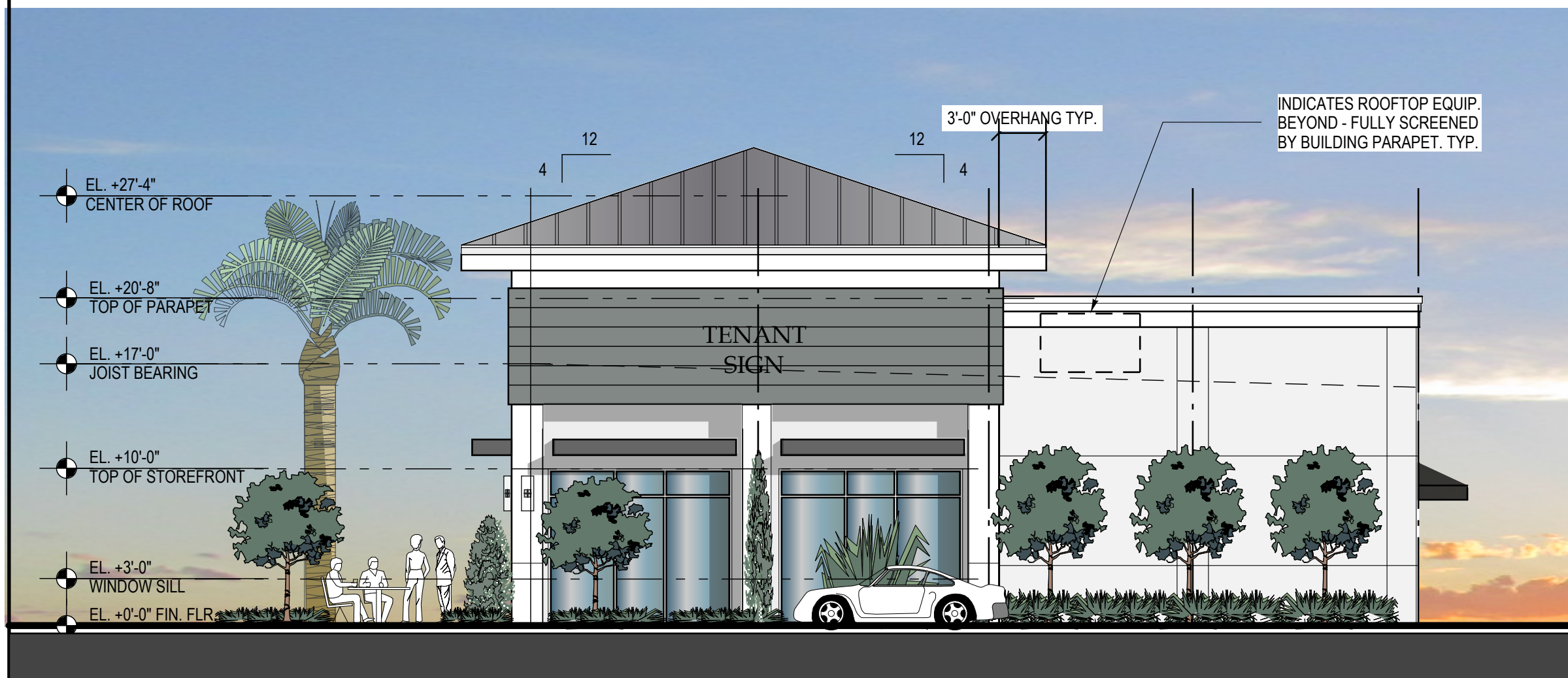
SIDE ELEVATION BUILDING #1 1/8" = 1'-0"
