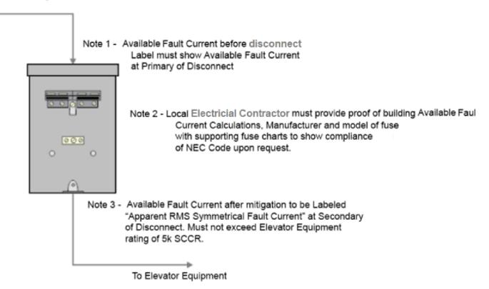
FIGURE 1: AVAILABLE FAULT CURRENT RATING LABELLING DIAGRAM
