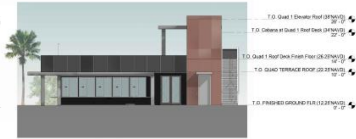
3 MAIN RESTAURANT SOUTH ELEVATION 1/8" = 1'-0"
