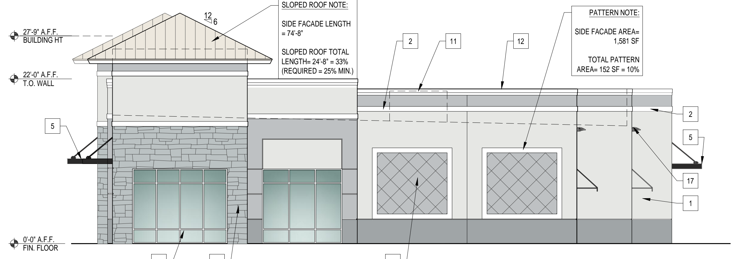
03 NORTH ELEVATION BUILDING 1 SCALE: 1/8" = 1'-0"
