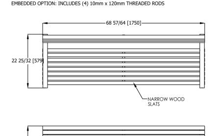
SURFACE MOUNT OPTION: (4) 1/4" THICK ANCHOR TABS WITH Ø1/2" HOLE FOR ANCHORING. NON-CORROSIVE ANCHORING
