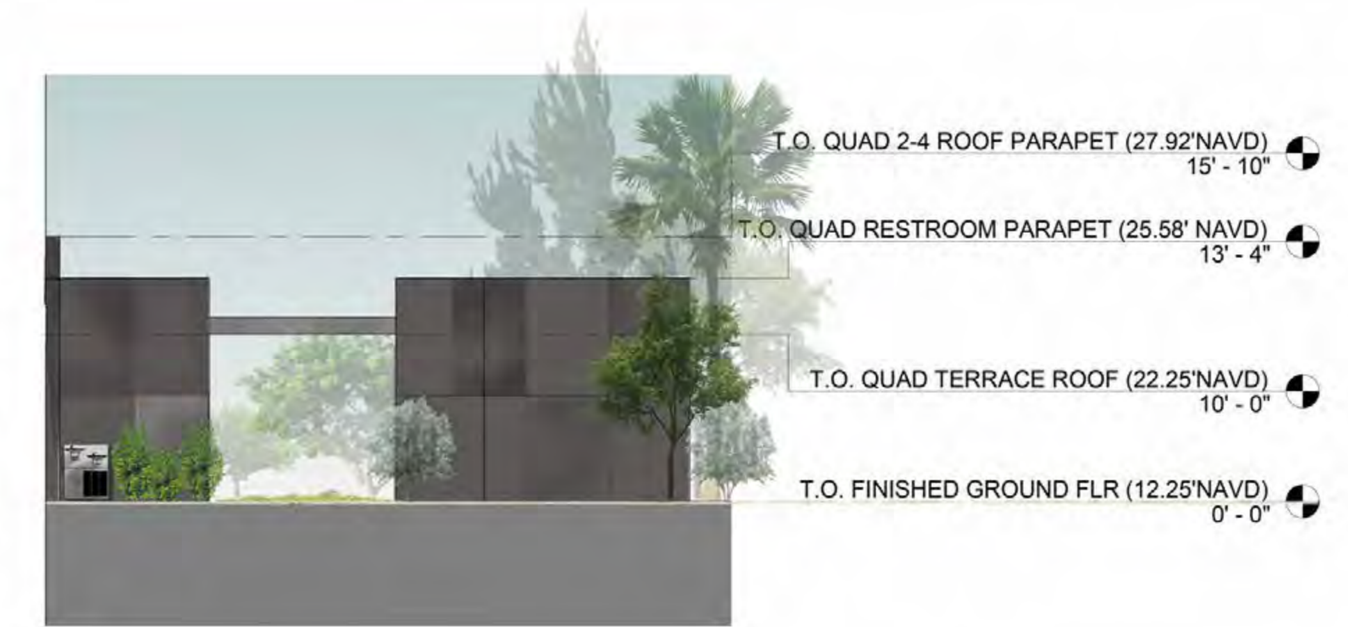
3 Quad 2 - WEST ELEVATION 1/8" = 1'-0"
