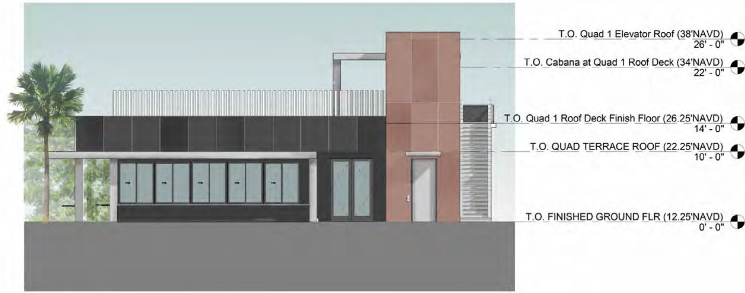
3 MAIN RESTAURANT SOUTH ELEVATION 1/8" = 1'-0"
