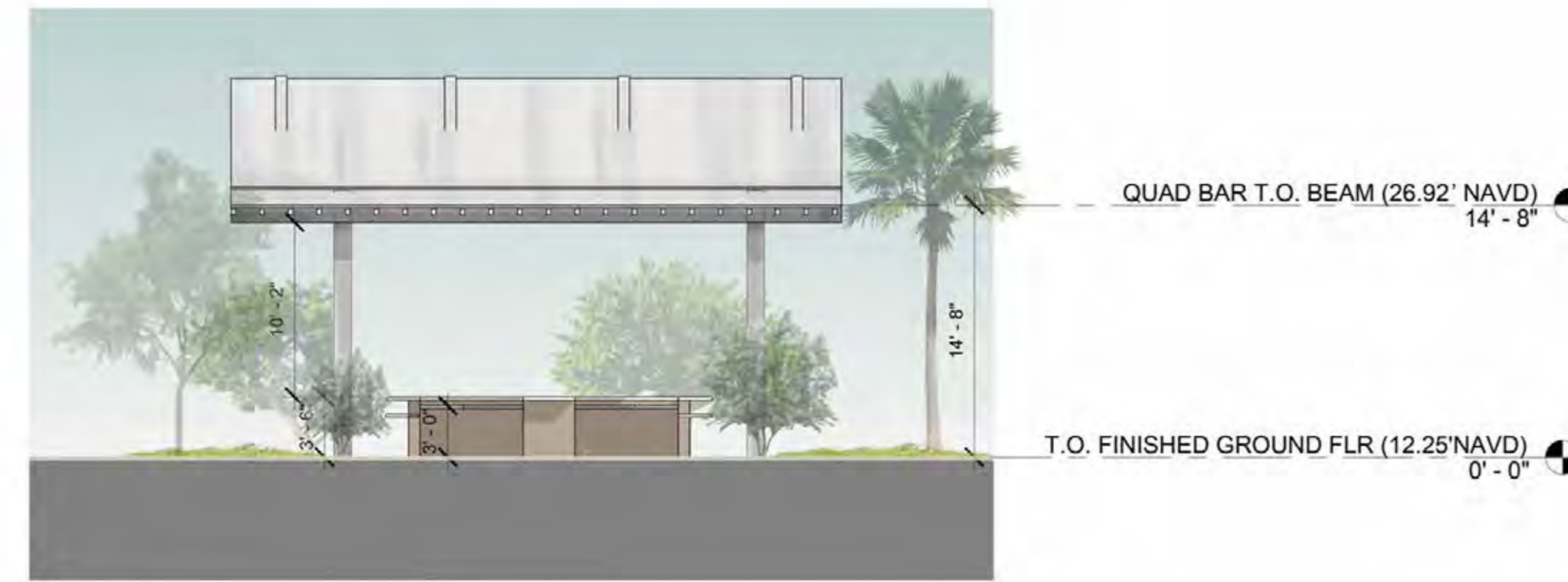
6 North Bar - SOUTH ELEVATION 1/8" = 1'-0"
