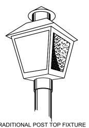
FPL TRADITIONAL POST TOP FIXTURE G.E. TC-100R LUMINARY WITH HIGH PRESSURE SODIUM LAMP ROUND, FIBERGLASS POLE, 12' HEIGHT (BURY 5' IN DEPTH).
