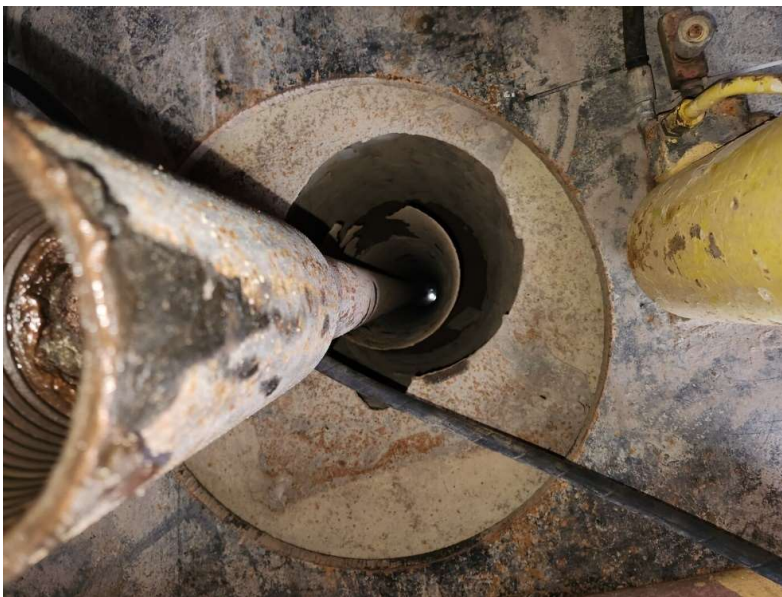
Photograph 2 – Drill pipe off center of inner steel casing
