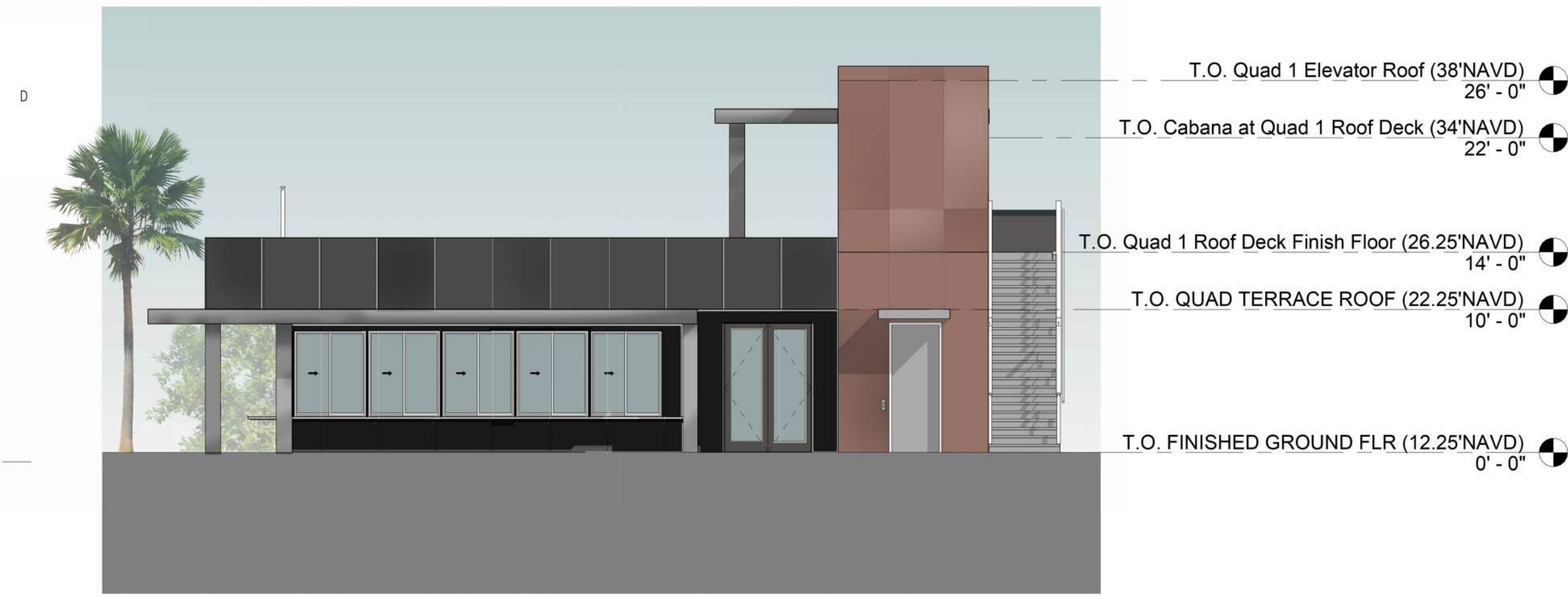
3 MAIN RESTAURANT SOUTH ELEVATION 1/8" = 1'-0"
