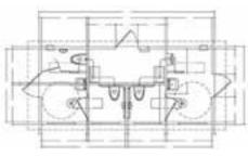
Dakota with chase restroom building. Standard features include simulated barnwood texture walls, simulated cedar shake textured roof, vitreous china fixtures, 4-gallon water heater, interior and exterior lights, off loaded, and set up at site.
