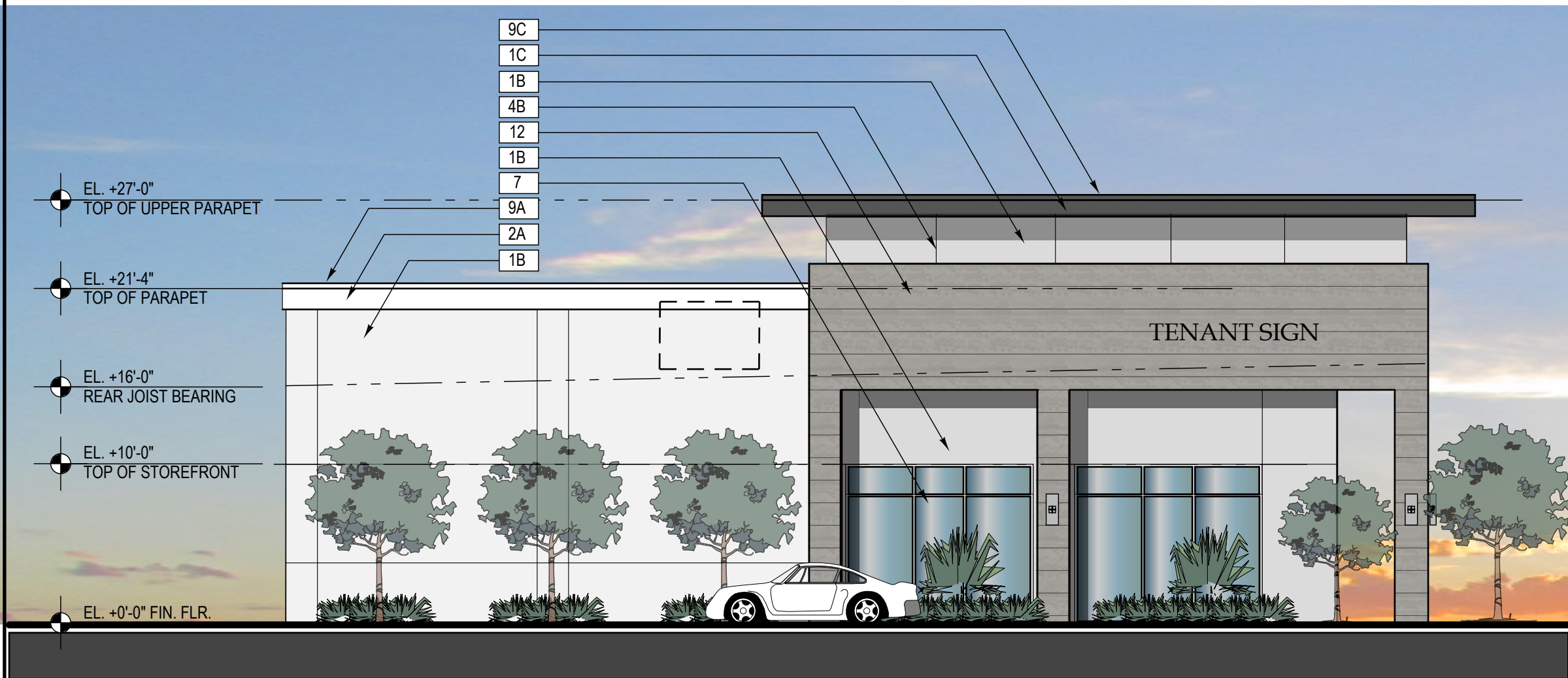
SIDE ELEVATION BUILDING #1 & #2 1/8" = 1'-0"
