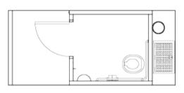
Gunnison single vault. Standard features include polyethylene lined concrete vault, barnwood textured walls, cedar shake textured roof, off loaded and set up at site.
