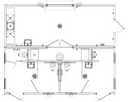
Keystone with chase restroom/concession building. Standard features include simulated barnwood texture walls, simulated cedar shake textured roof, interior and exterior lights, vitreous china fixtures in restroom, 30-gallon water heater, three compartment stainless steel sink in concession area, roll up concession window, off loaded and set up at site.
