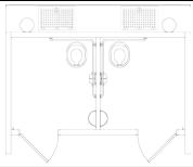
Double Cascadian double vault. Standard features include two polyethylene lined concrete vaults, board and batt upper and lap siding lower textured walls, cedar shake textured roof, off loaded and set up at site.
