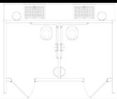
Tioga Special double vault. Standard features include two polyethylene lined concrete vaults, barnwood textured walls, cedar shake textured roof, off loaded and set up at site.
