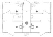
Montrose with chase restroom building. Standard features include simulated barnwood texture walls, simulated cedar shake textured roof, vitreous china fixtures, 30-gallon water heater, interior and exterior lights, off loaded, and set up at site.
