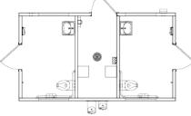
Ozark II with chase restroom building. Standard features include simulated barnwood texture walls, simulated cedar shake textured roof, vitreous china fixtures, 4-gallon water heater, interior and exterior lights, off loaded, and set up at site.
