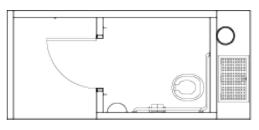
Rocky Mountain single vault. Standard features include polyethylene lined concrete vault, board and batt upper and rock lower textured walls, cedar shake textured roof, off loaded and set up at site.
