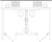
Double Rocky Mountain double vault. Standard features include two polyethylene lined concrete vaults, board and batt upper and rock lower textured walls, cedar shake textured roof, off loaded and set up at site.
