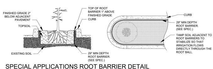
2- ROOT BARRIER SHALL BE INSTALLED PER MANUFACTURER'S SPECIFICATIONS AND RECOMMENDATIONS
