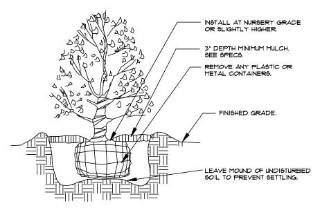
\* SEE SPECIFICATIONS FOR BACKFILL MIXTURE AND FERTILIZATION.
