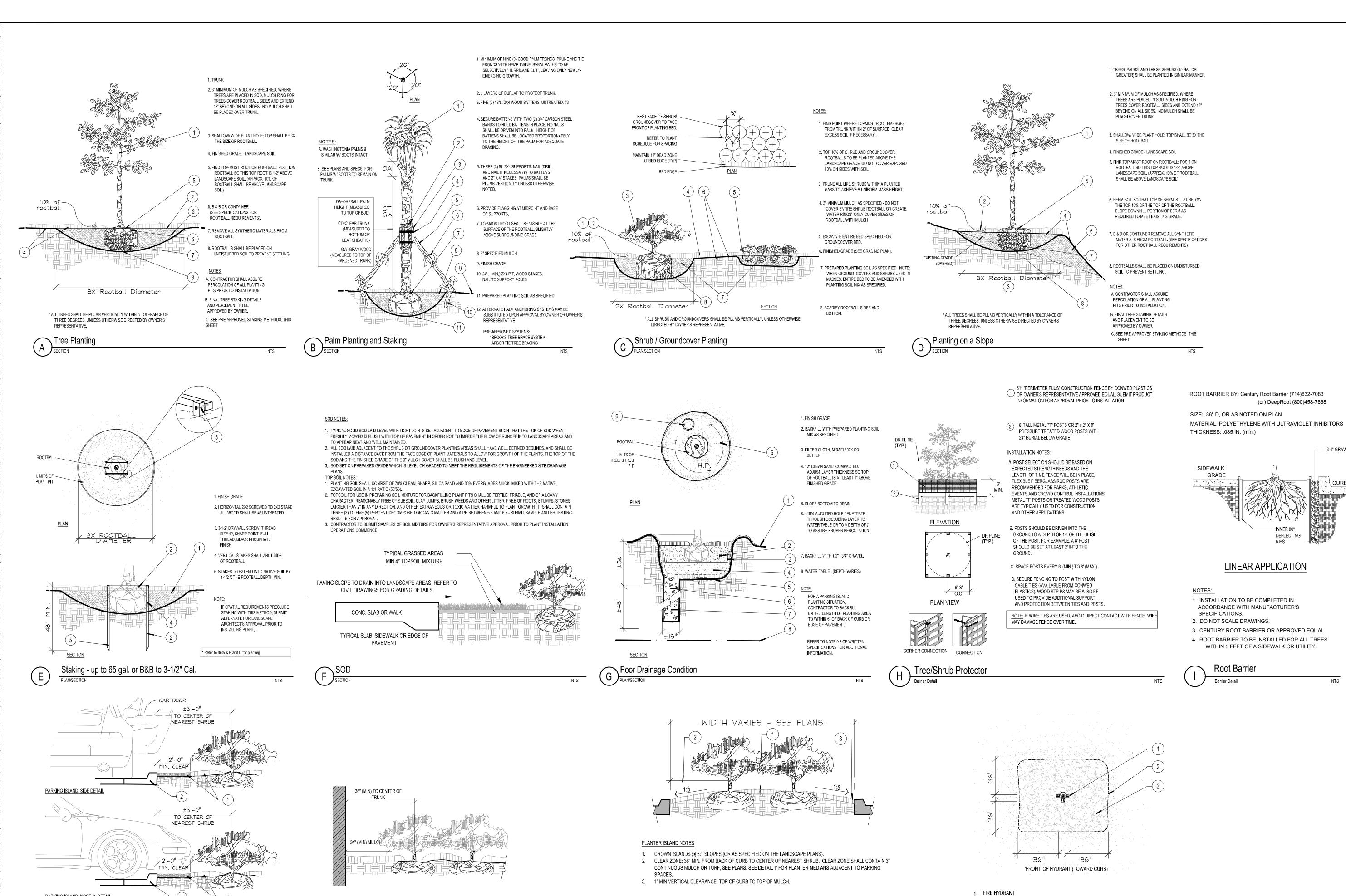
EXCAVATE CONTINUOUS 36" DEEP (FROM TOP OF CURB) FOR ENTIRE LENGTH AND WIDTH OF ISLAND &
