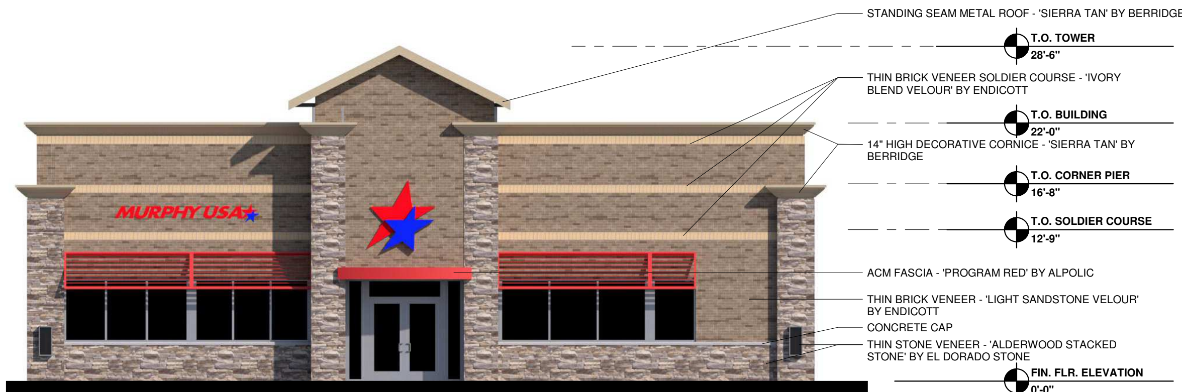
5 ELEVATION - FRONT BUILDING ONLY (FACING WEST)
