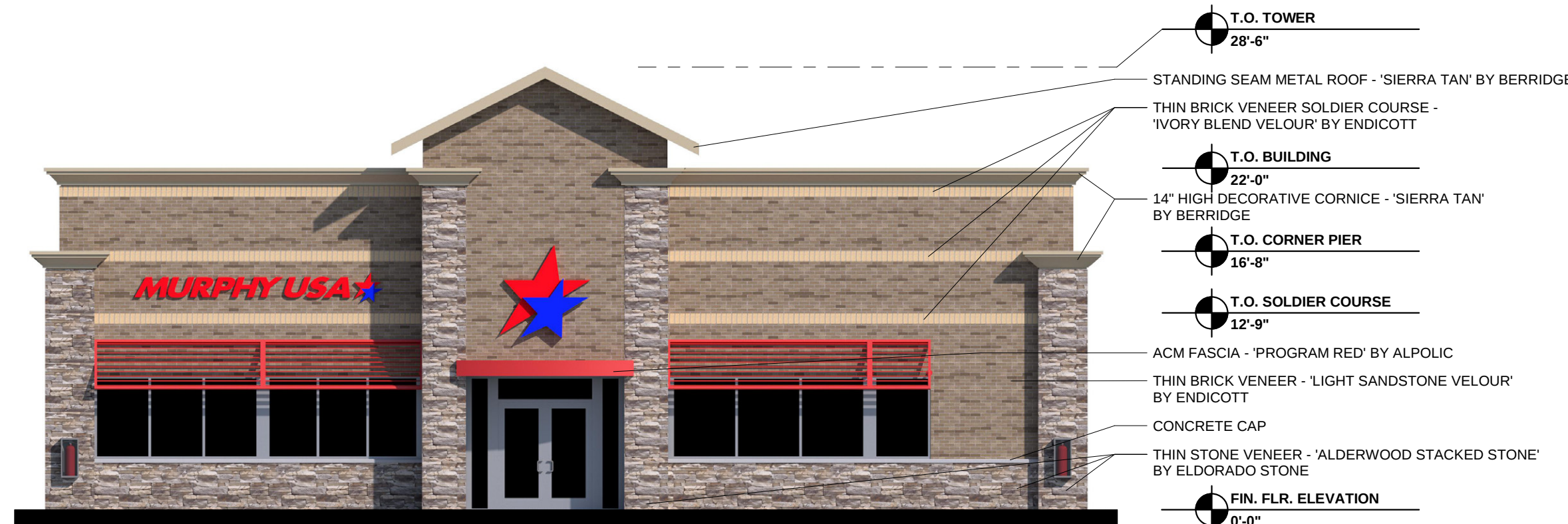
5 ELEVATION - FRONT BUILDING ONLY (FACING EAST)
